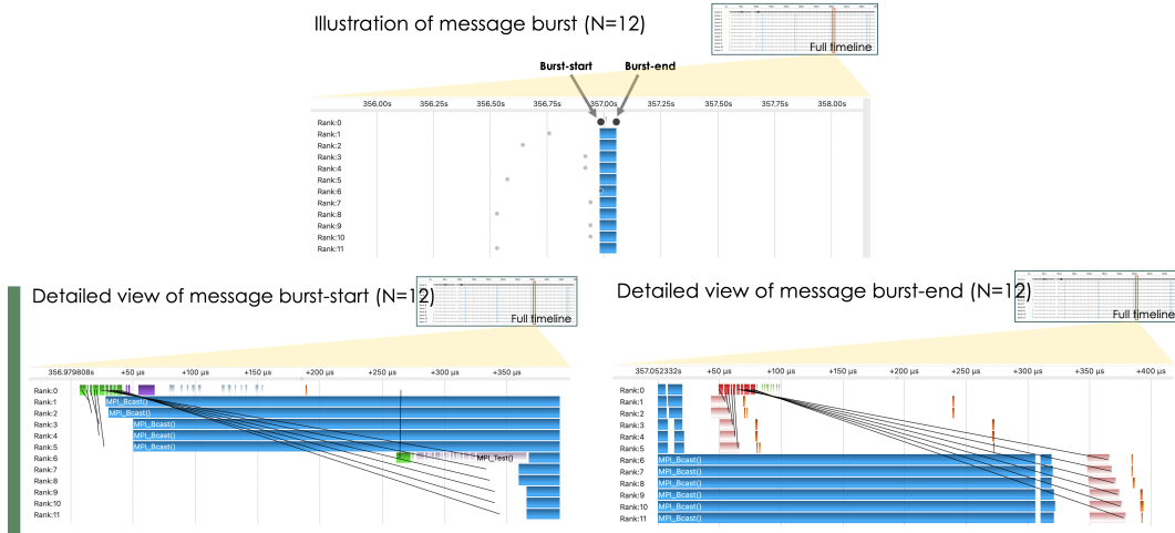
Figure 29: Message burst and communication pattern for N = 12
